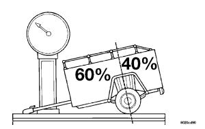
Trailer sway control and equalizing hitch are required for tongue weights above 350 lbs. (159 kg).
